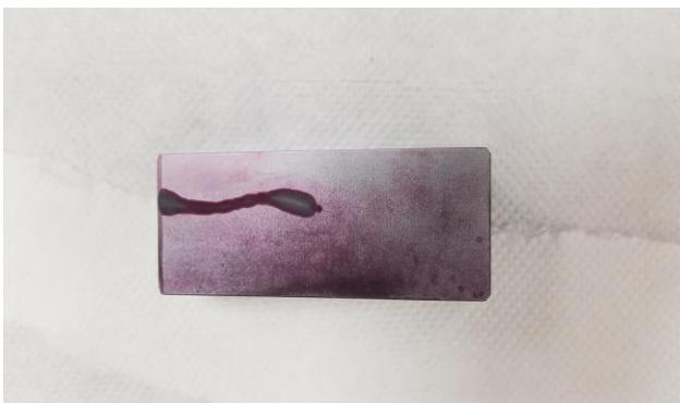
**Fig. 3. Photographic record from NDT control by PT method**
