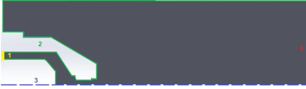
**Fig. 6. Boundaries for the simulation of flow: 1 – flow input, 2 – impenetrable walls, 3 – axes of symmetry, 4 – flow output**
