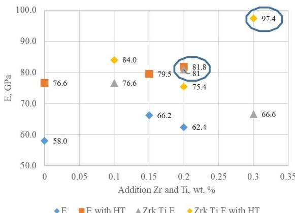
**Fig. 5. Dependence of  $E$  before and after HT for investigation alloys AlSi7Mg0.3Cu**
