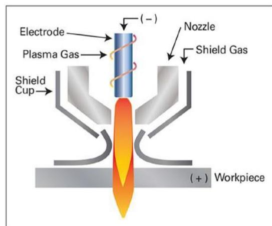
Fig. 1. The plasma arc cutting process [1]
