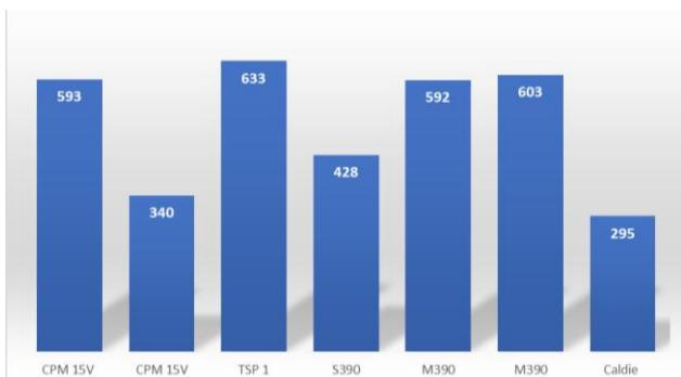
Fig. 10. Maximum measured value of the nitriding layer thickness of the samples [µm]
