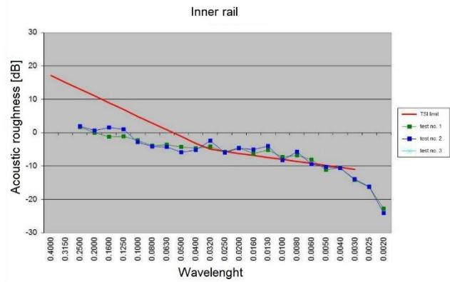
Fig. 2. Acoustic roughness of the inner rail
