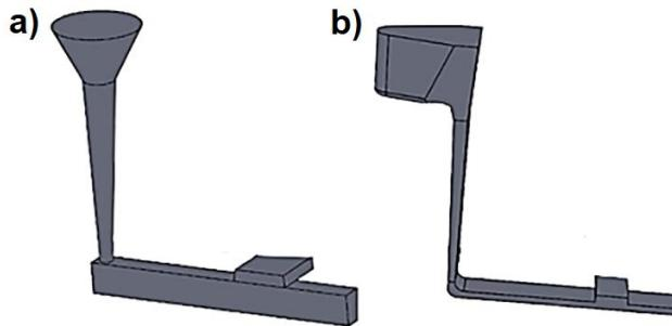
**Fig. 2.** Gating system design for numerical simulation:
