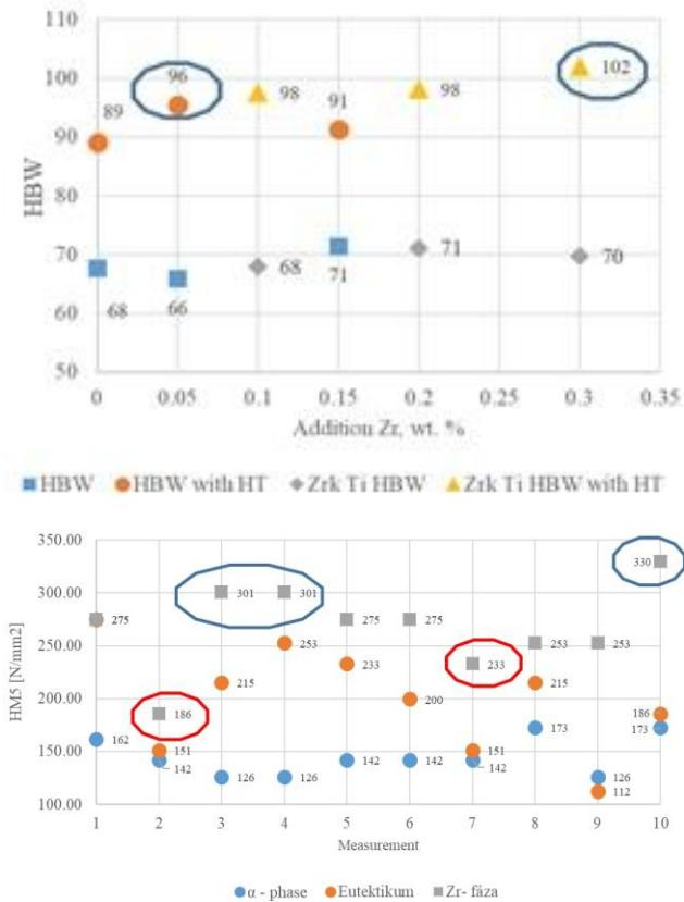
Fig. 7. HBW for investigation alloys AlSi7Mg0.3Cu and *HMS* microhardness for *E3* alloy
