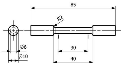
**Fig. 1. Scheme of the test specimen**
