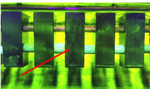
**Fig. 5. Photographic record from MT with shown inhomogeneity**
