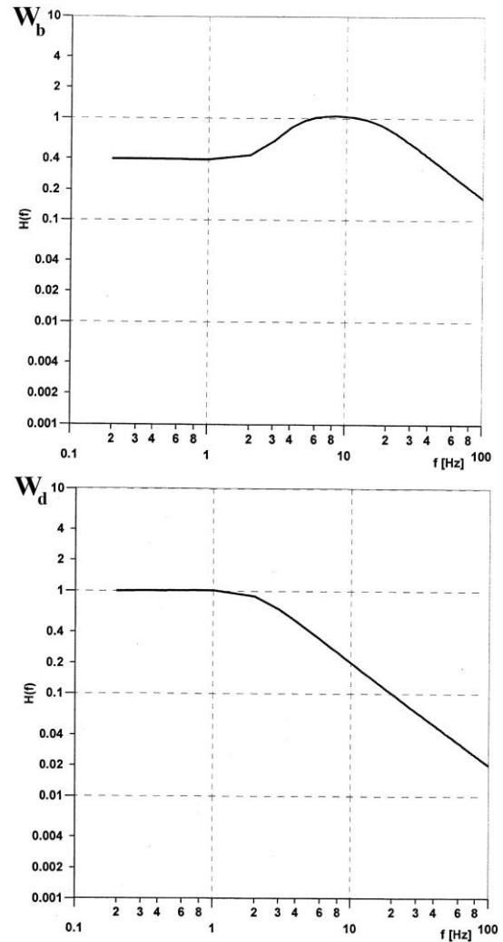
**Fig. 3. Weighed functions  $W_b$  and  $W_d$**
