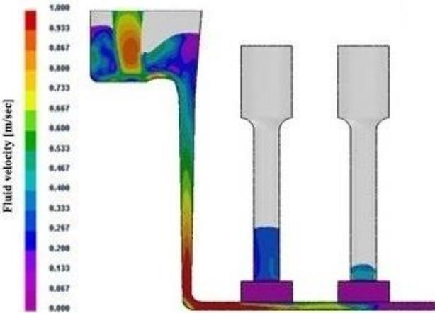
**Fig. 7. Analysis of the fluid velocity in the naturally pressurized gating system with filter media**
