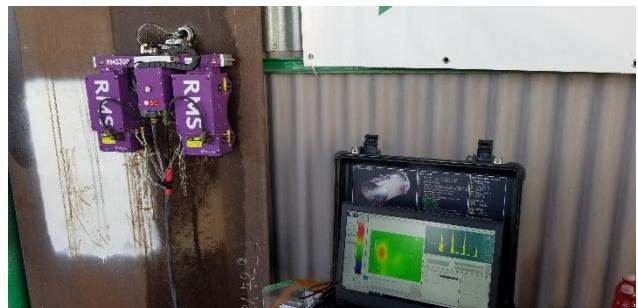
**Fig. 2. Ultrasonic (conventional) corrosion mapping system.** Useful to inspect walls of storage tanks to size the remaining wall thickness, but also to detect material changes by selecting the attenuation option interpretation for scanned data. Can work through coatings.
