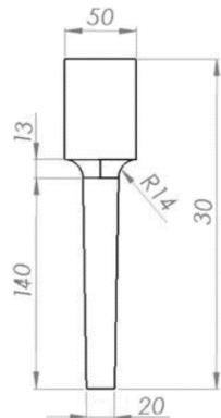
**Fig. 3.** Design of casting
