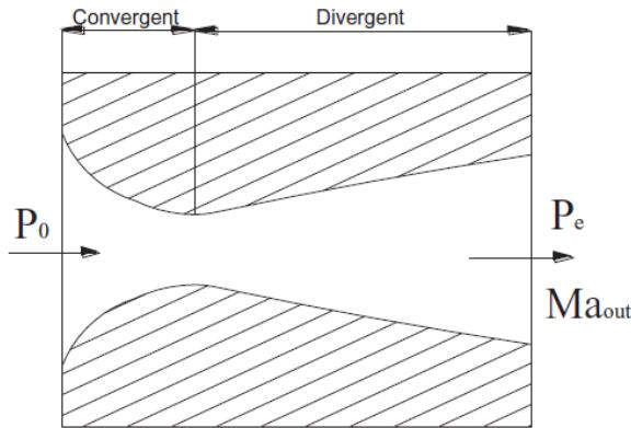
**Fig. 2. Structure of the Laval nozzle [7]**
