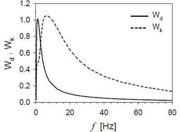
Fig. 1. Boundaries of reduced comfort (dash line), limit of reduced performance (solid line) for effective values of accelerations in the third octave band for horizontal direction
