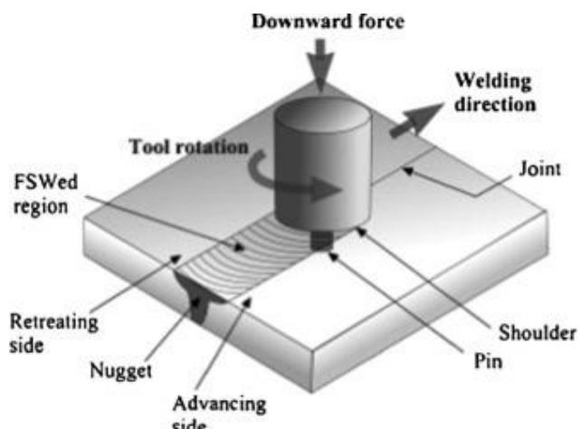
Fig. 1. Schematic drawing of FSW process [2].
