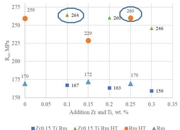
**Fig. 3. Dependence of  $R_m$  before and after HT for investigation alloys AlSi7Mg0.3Cu**
