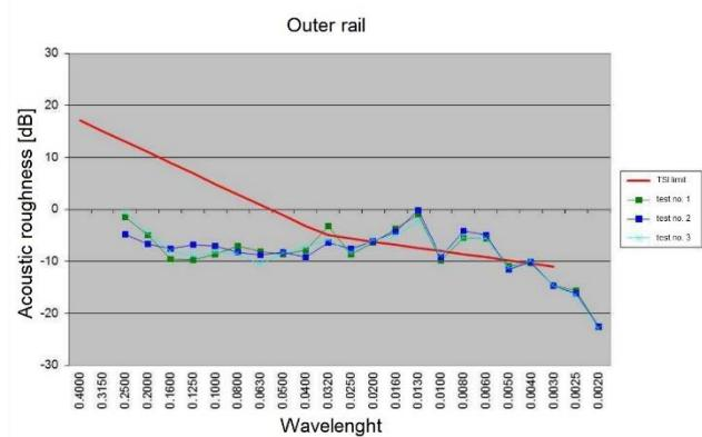
Fig. 3. Acoustic roughness of the outer rail
