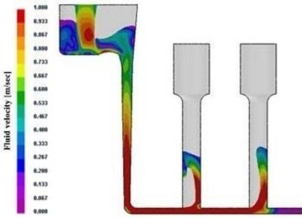
**Fig. 6. Analysis of the fluid velocity in the naturally pressurized gating system without filter media**
