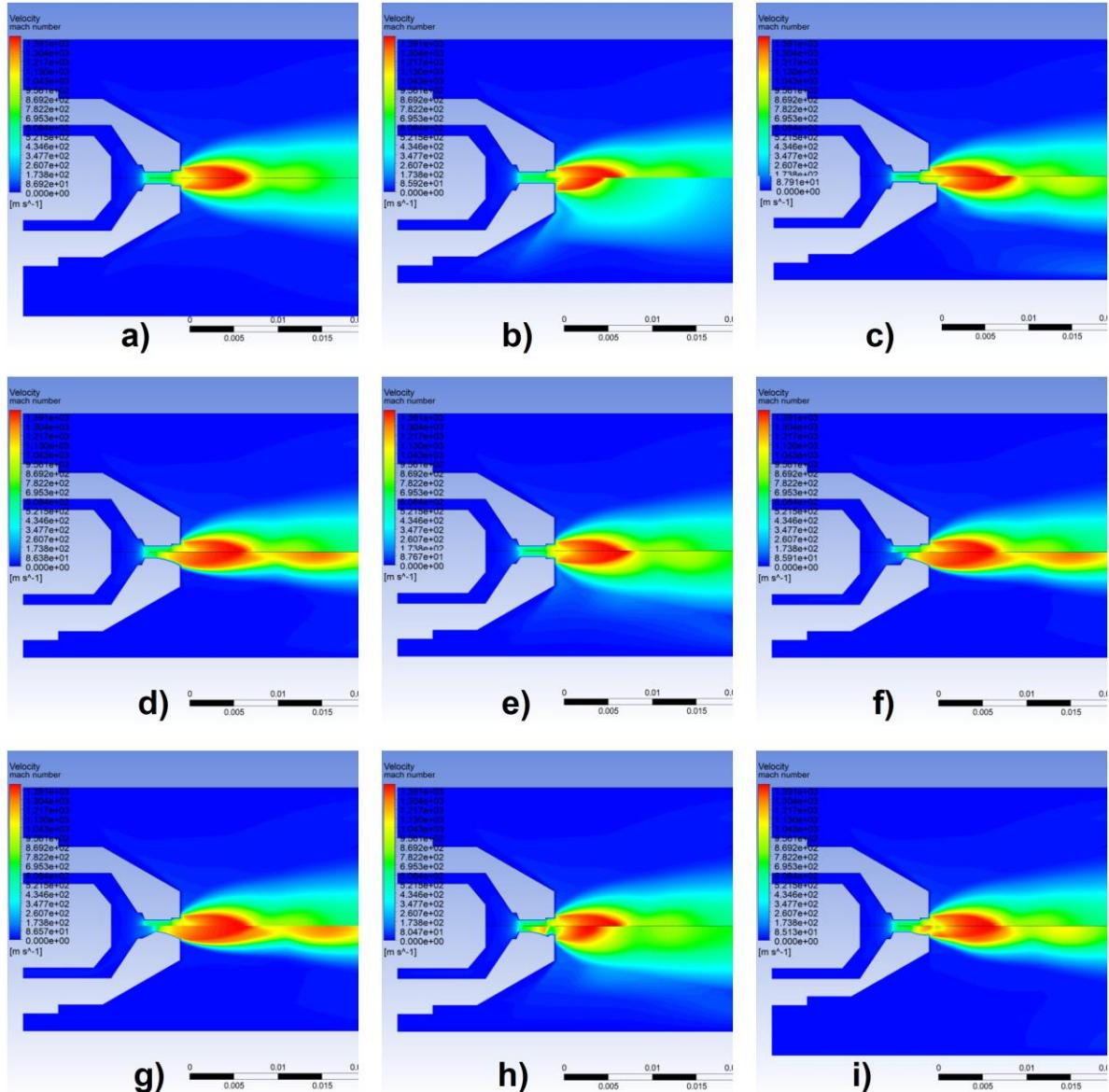
**Fig. 8. Results of comparison of flow simulation: a) reference nozzle; b) to i) modified nozzles (upper half of picture is reference nozzle and lower half is modified nozzle)**
