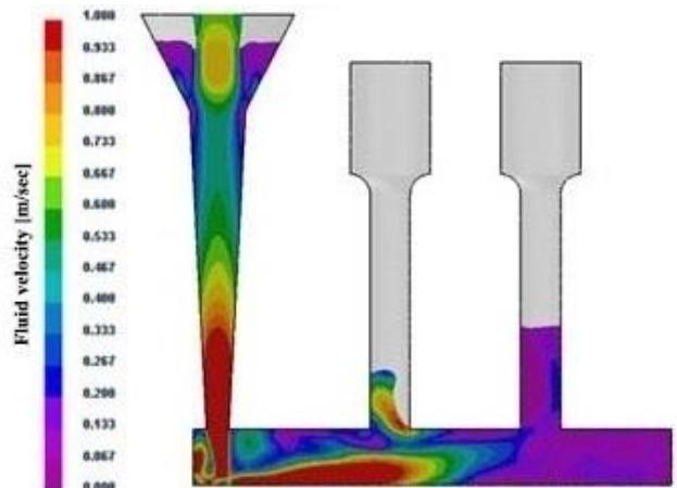
**Fig. 4.** Analysis of the fluid velocity in the non-pressurized gating system without filter media
