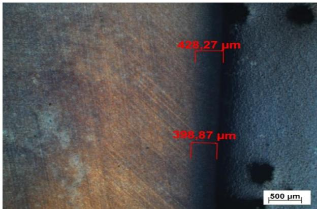
Fig. 4. Nitriding layer thickness S390
