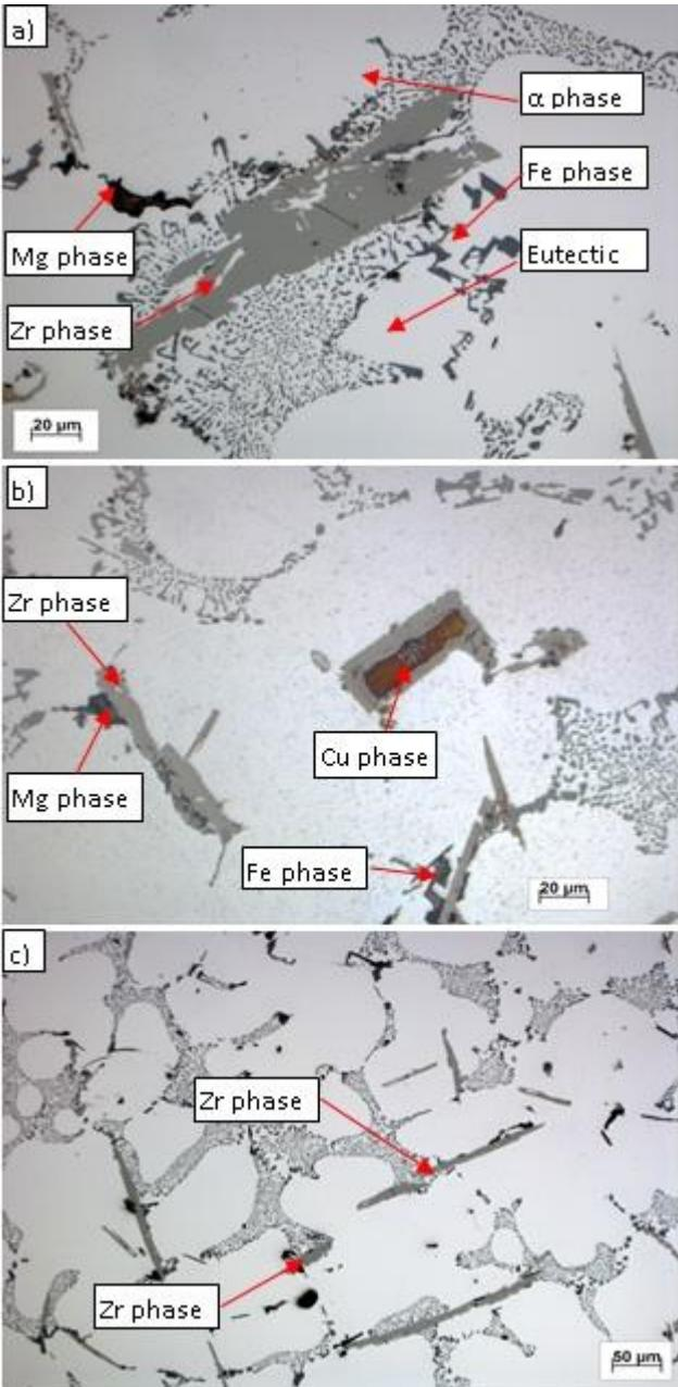
**Fig. 9. Microstructure of the alloys before HT:** a) R alloy, b) E1 alloy, c) E2 alloy,  $\text{H}_2\text{SO}_4$  etch
