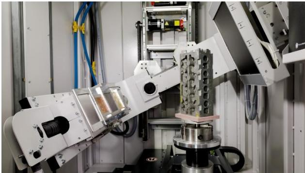
**Fig. 5. Automated high-resolution CT inspection system in Automotive industry.** Detects defects over the defined level of threshold. Can be used also for dimensional analysis. Can be combined with the conveyor belts and robotic arms to sort OK and NO OK parts. X-Ray cabinet solution [6].
