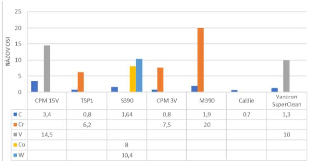
Fig. 8. Comparison of chemical composition [%]
