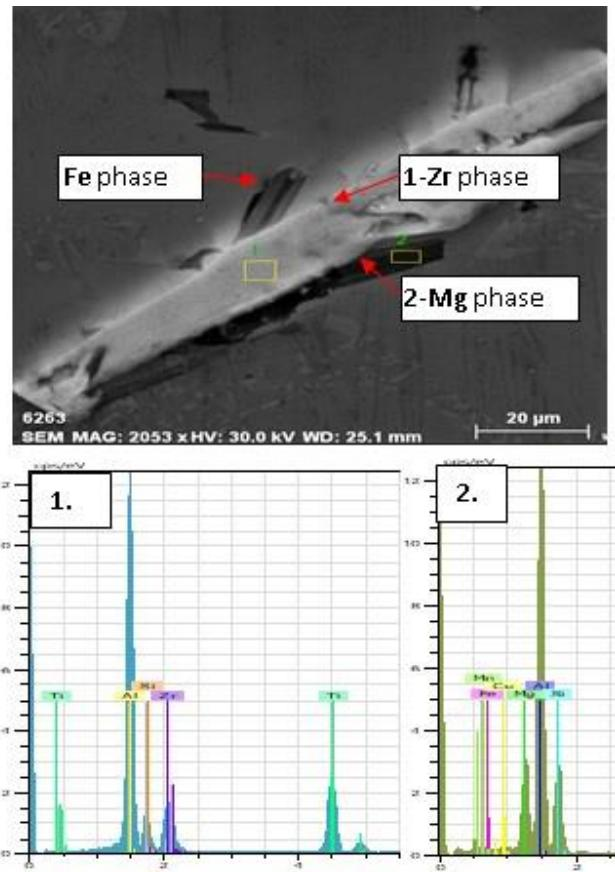
Fig. 8. EDX analysis of the Zr phase in the AlSi7Mg0.3CuZr0.15 *R* alloy
