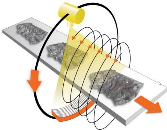
**Fig. 4. Automated CT inspection system in Automotive industry.** Detects defects over the defined level of threshold. Can be used also for dimensional analysis. Can be combined with the conveyor belts and robotic arms to sort OK and NO OK parts [6].
