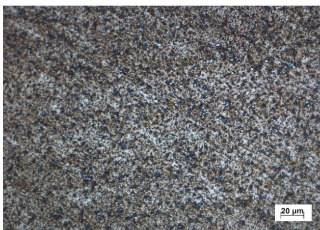
Fig. 1. Microstructure after nitriding (incr. 1000x) CPM 3V
