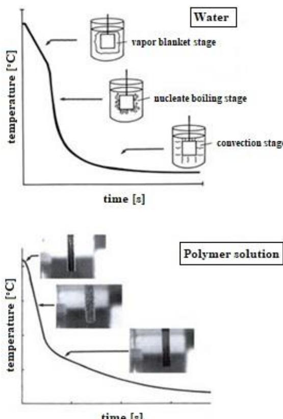
**Fig. 3. Water and polymer solution cooling process [8]**
