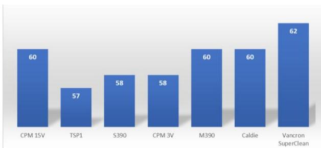
Fig. 9. Average hardness of samples [HRC]
