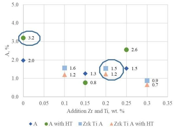
**Fig. 6. Dependence of  $A$  before and after HT for investigation alloys AlSi7Mg0.3Cu**
