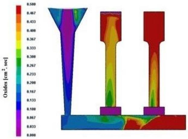
**Fig. 9. Analysis of the amount of oxides in the non-pressurized gating system with filter media**
