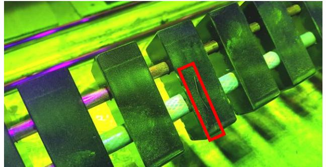
**Fig. 6. Photographic record from NDT control by MT method**
