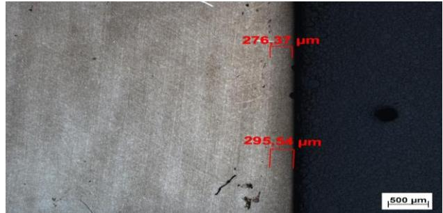
Fig. 6. Nitriding layer thickness CALDIE
