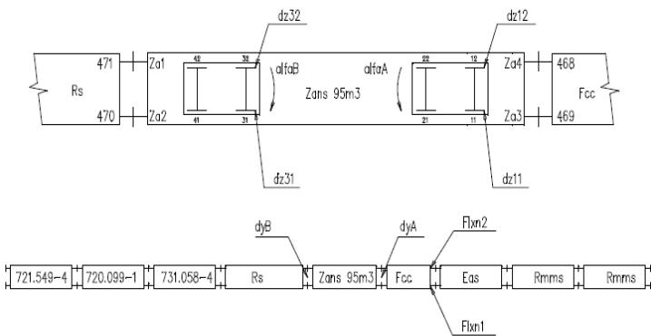
**Fig. 3. Scheme of test set and measuring points**
