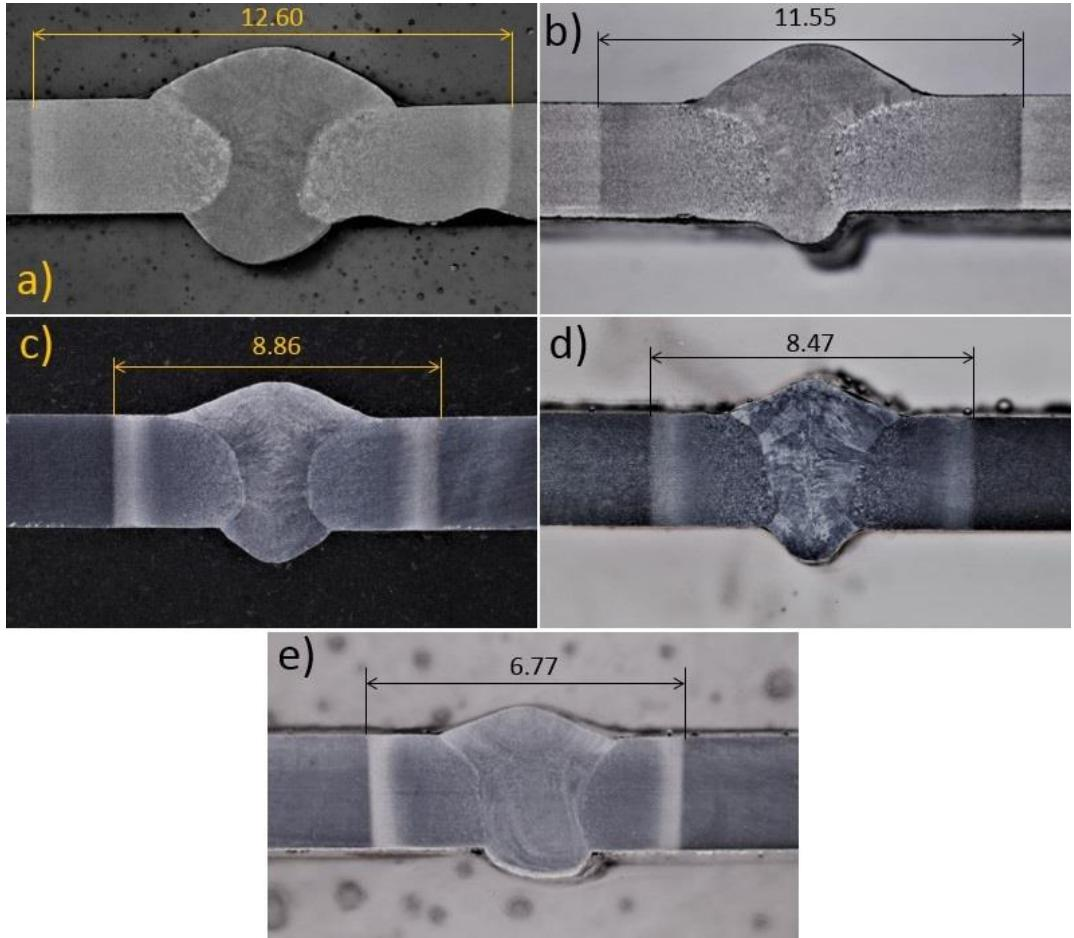
**Fig. 2.** Cross-sectional images of investigated welds welded by various methods: a) 135 – short arc, b) 135 – pulsed, c) 135 – CMT, d) 138 – short arc, e) 138 – short arc (cooled)
