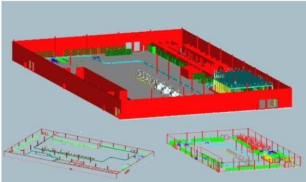
**Fig. 5. 3D layout of production systems with logistics areas and tracks**
