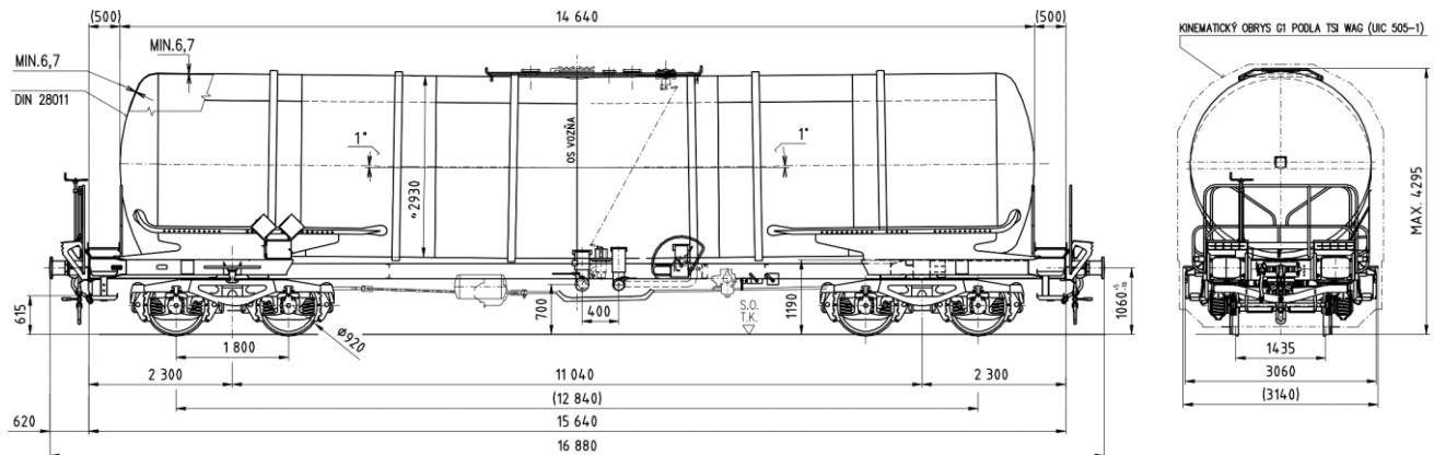
Fig. 1. Scheme of the tested tank wagon Zans 95 m<sup>3</sup>
