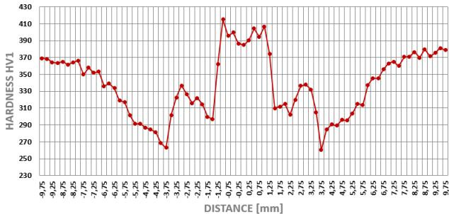
Fig. 4. Cross-sectional hardness distribution on FCAW welded joint in short arc mode
