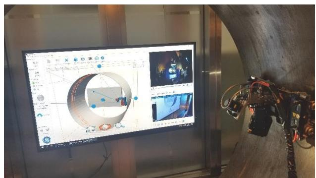
**Fig. 3. RVI system used to inspect inner parts of the storage tanks.** Combined with the laser system and CAD drawing, system knows and remembers position of robot, but also the position of viewed area. Data are automatically recorded so the operator next time just send the unit to selected position to compare the changes if any.
