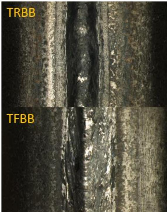
Fig. 1 Detailed images of the specimens after the bending test
