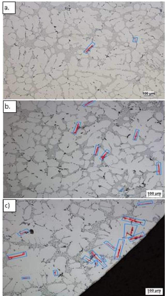
**Fig. 10. Microstructure of E1, E2, and E3 alloys before HT:** a) 0.1 wt.%  $Ti$ , b) 0.2 wt.%  $Ti$ , c) 0.3 wt.%  $Ti$ ,  $\text{H}_2\text{SO}_4$  etch
