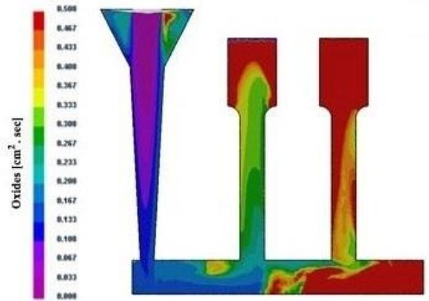
**Fig. 8. Analysis of the amount of oxides in the non-pressurized gating system without filter media**
