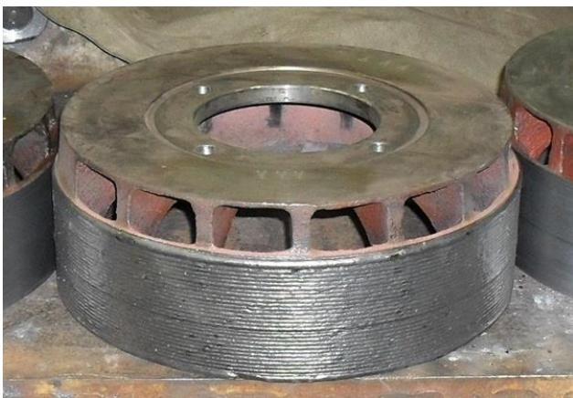
Fig. 2. Surface of freshly welded brake drum
