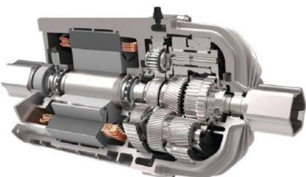
Obr. 7. E-axle spoločnosti Schaeffler [16]
