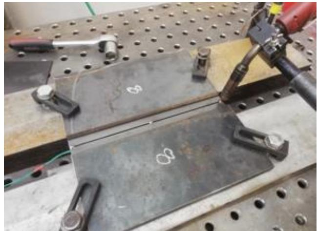
**Fig. 1. Welded parts clamped on the working table**
