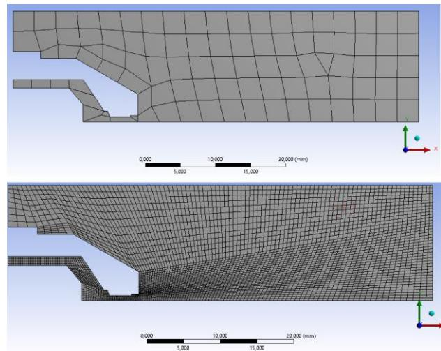
**Fig. 5. Comparison of an automatically generated mesh and an adjusted mesh**
