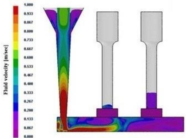
**Fig. 5.** Analysis of the fluid velocity in the non-pressurized gating system with filter media
