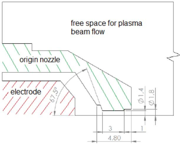
**Fig. 3. A 2D schematic model of a nozzle with an electrode for simulation of a plasma flow**
