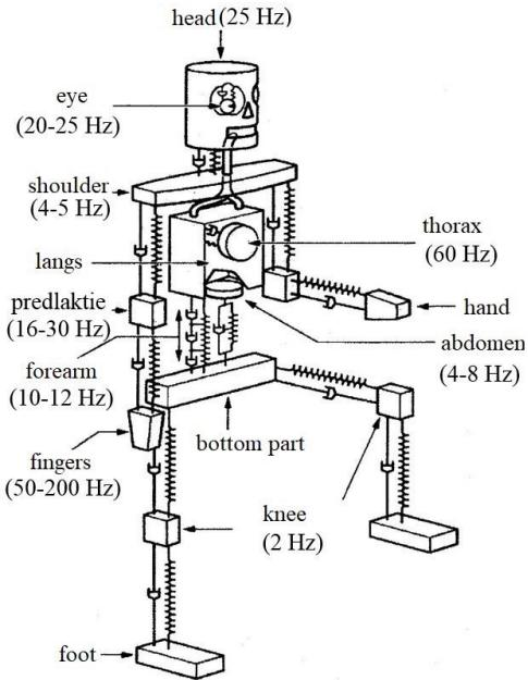
Fig. 1. A dynamic model of a human body
