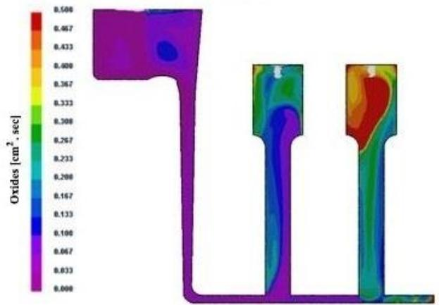
**Fig. 10. Analysis of the amount of oxides in the naturally pressurized gating system without filter media**
