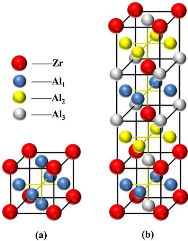
**Fig. 1.** Al<sub>3</sub>Zr phase crystallographic lattices: a) L<sub>12</sub> b) DO<sub>23</sub>
