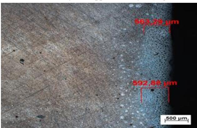
Fig. 5. Nitriding layer thickness M390
