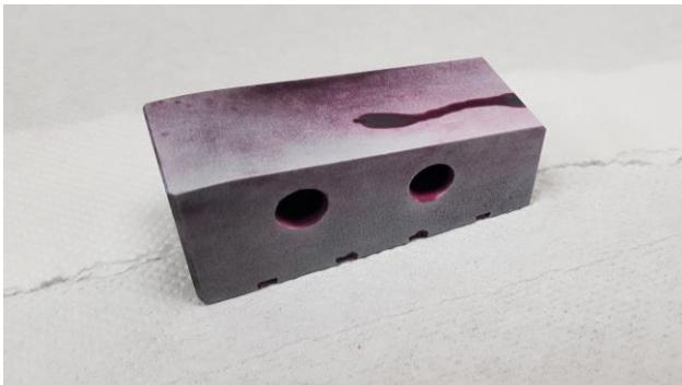
**Fig. 4. Representation of the error by PT, evaluation after 5 min.**
