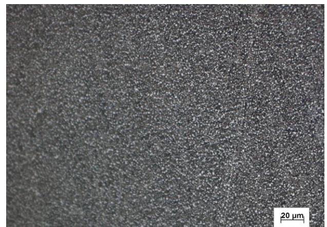
Fig. 7. Microstructure after nitriding (incr. 1000x) Vancron SuperClean
