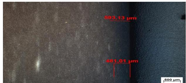
Fig. 2 Nitriding layer thickness CPM 15V.
