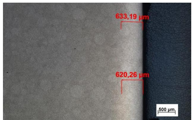
Fig. 3. Nitriding layer thickness TSP1
