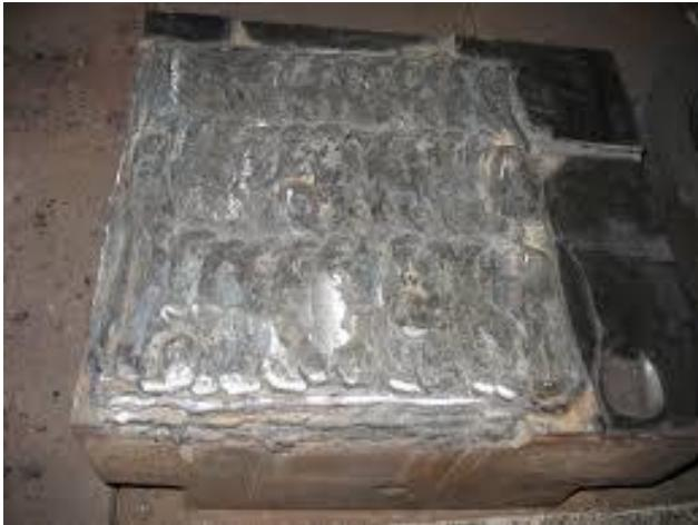
Fig. 1. Renovation of flat surfaces - die welded by method 136
