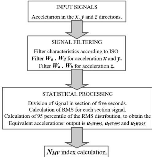
**Fig. 4. Procedure of processing and calculation of ride comfort index**
