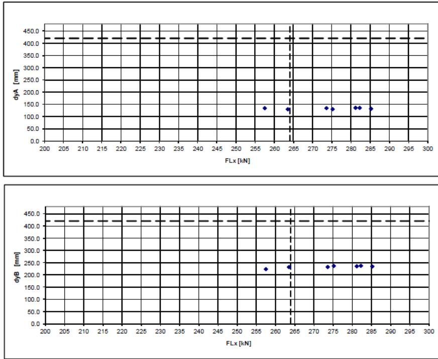
**Fig. 5 Dependence of mutual transverse displacements of buffer heads on longitudinal tractive force**
