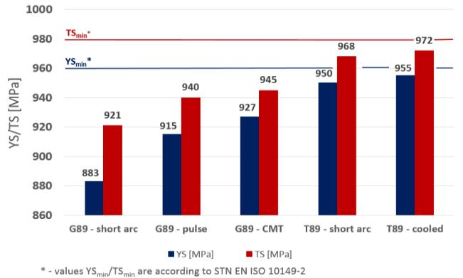
**Fig. 3. YS/TS values for various welding parameters**
