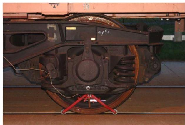
**Fig. 2. Sensor of wheel lift**
