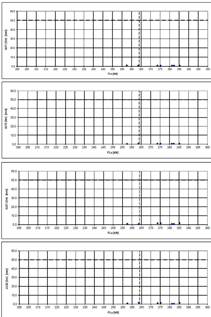
**Fig. 4 The dependence of the wheel lift on the longitudinal tractive force at the inner rail of the curve**
