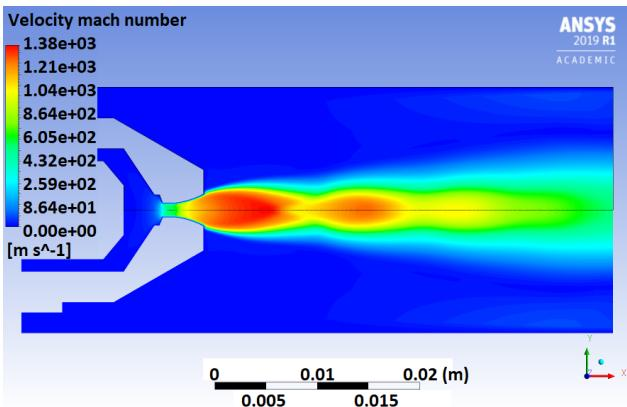
Fig. 9. Modified nozzle No. 7 flow simulation
