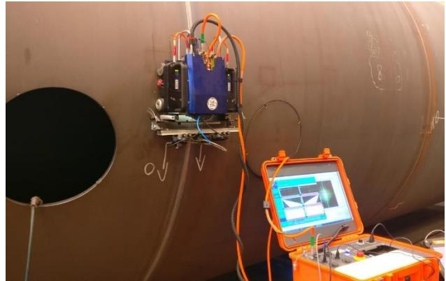
**Fig. 1. Ultrasonic Phased Array Inspection System** - Inspection of LPG pressure tanks with the automated weld laser following, to maintain the proper distance of the probes from the weld. System scanning speed depends on the selected UT hardware. Can be adjusted from  $1 \text{ cm} \cdot \text{s}^{-1}$  up to  $5 \text{ cm} \cdot \text{s}^{-1}$ . Such system can reduce the inspection time almost by 75 % compared to X-Ray inspection, thus speeding up the production process.
