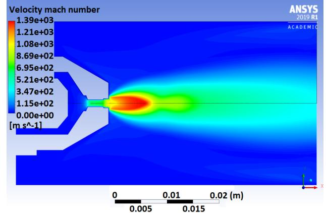
**Fig. 7. Reference nozzle flow simulation**
