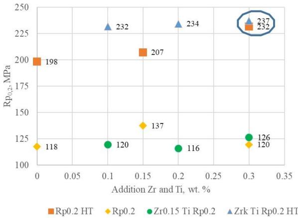
**Fig. 4. Dependence of  $R_{p0.2}$  before and after HT for investigation alloys AlSi7Mg0.3Cu**
