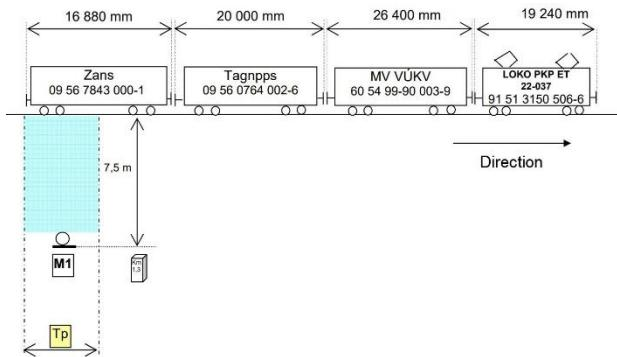
Fig. 1. Composition and orientation of the test set
