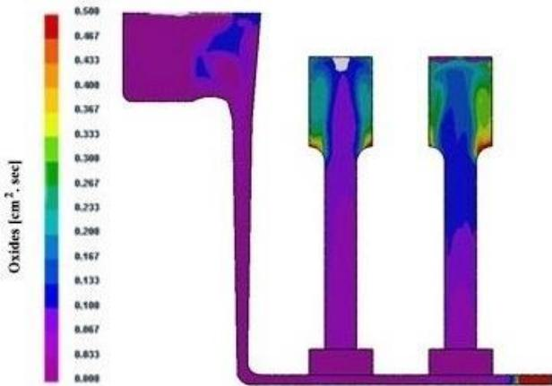
**Fig. 11. Analysis of the amount of oxides in the naturally pressurized gating system with filter media**
